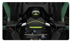
Hydraulic Steering Damper and Redesigned Steering Column An industry first, it redefines rider control by reducing input from the water; creating a solid and predictable feel that can be adjusted to rider preference. A reinforced steering column will withstand high performance stress.
